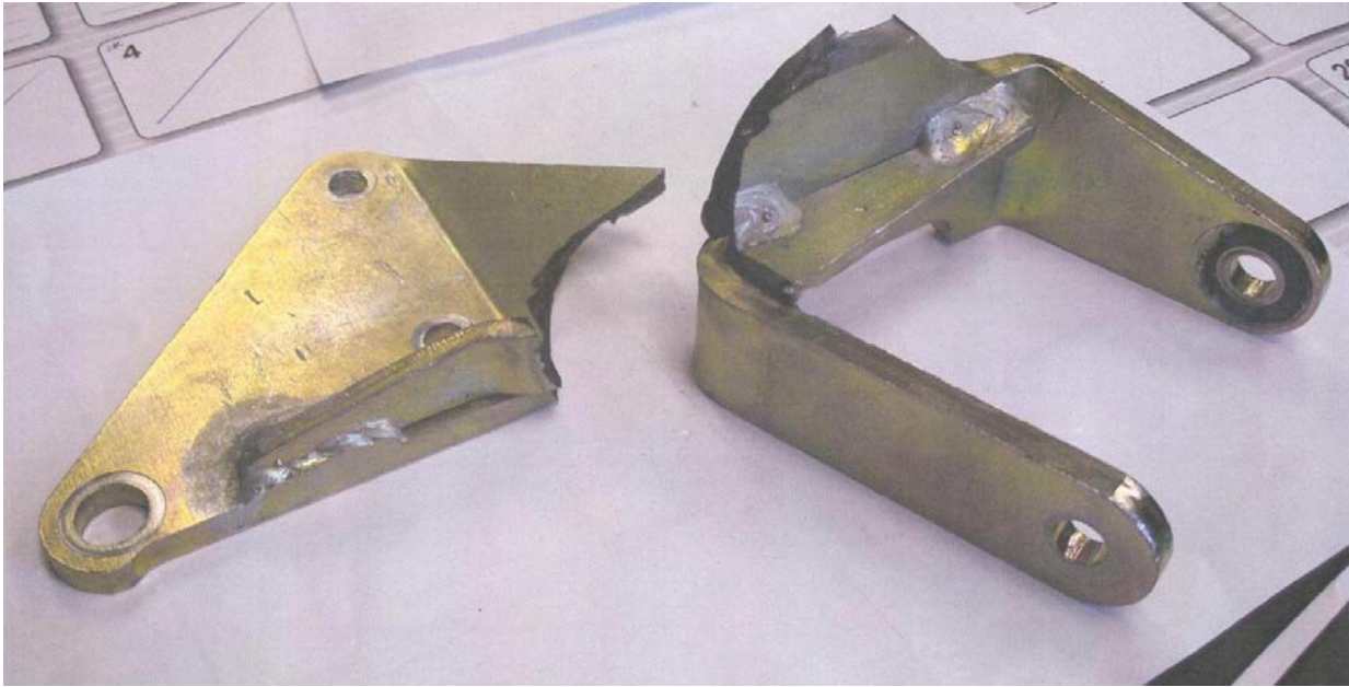
Figure 1 Broken Alternator Bracket
